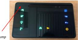
Control button to switch on the electric power supply for the pump
