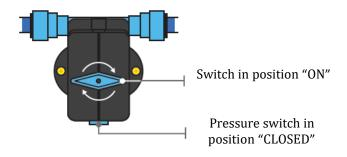
Turn on the pump at the control panel.
