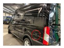
For supplying your vehicle with 230 V, the vehicle must be connected via a standard CEE-coupling outside on the rear left-hand side of the vehicle.
