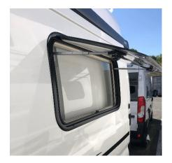
To close the window, open the lever to the stop and then lower it.
