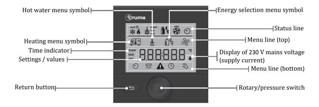
Different values and parameters can be selected, changed and stored with the rotary/pressure switch. The selected menu items flash.
