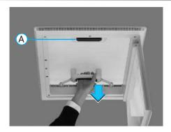
Before opening the roof hatch, first open the insect grille. In order to push up (and close) the hatch, handle lock A must be pressed in. The roof hatch can be closed at each side. The insect grille can be removed for cleaning. Pull down grille and pull off.
