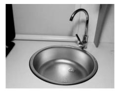
The sink of your Karmann motorhome is supplied with a mixer tap, which functions like a standard household tap. However, first make sure that the pump switch is on (see control panel, Page 6-1).
