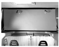
The floor of the overcab bed can be folded up by 90 degrees to permit convenient access to the driver's cabin.
