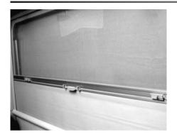
All windows are provided with a shade and insect blind. The illustration shows both blinds in half-open position. Both blinds can be pushed up and down together or separately.
