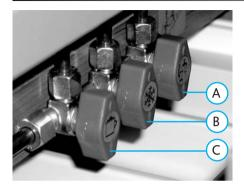
where the distributor is installed horizontally, they are open in vertical position. All gas devices are doubly secured. Please also note the attached operating instructions. If you do not use your motorhome for several days, you should always close your gas cylinders.
