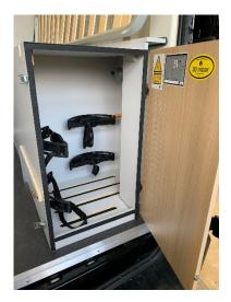
Before shut-down for a longer period of time, it is highly recommended to disconnect the gas cylinders and to store them in a well ventilated place.
