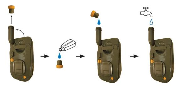
**Note:** In very warm weather or prolonged storage, more WC fluid may have to be used. For best results, use only fluids intended for Thetford toilets. Do not leave any residual amounts in the tank when shutting down for winter.
