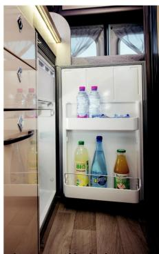
The cooling power depends on the ambient temperature, the amount of food to be kept cool and the number of times the refrigerator door is opened.
