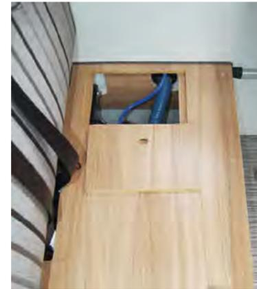
Your mobile home is equipped with a fixed fresh water tank with a capacity of 80 L. The tank is located underneath the left bench, behind the driver's seat.
