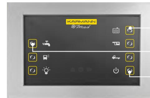
Control light for fresh water tank filling level
