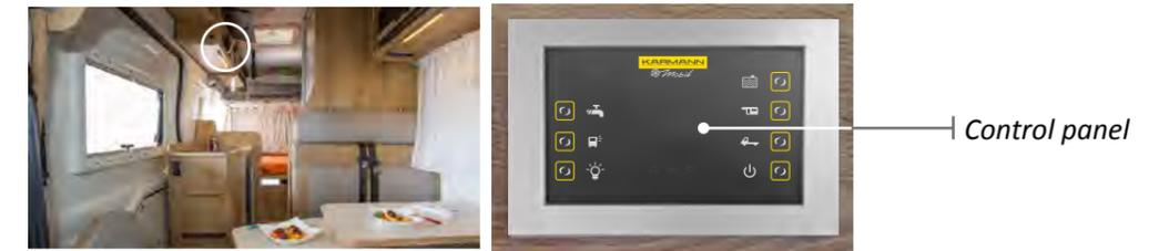
The control panel allows you to control various electric appliances in your vehicle and to check several parameters for the optimal use of the living room.
