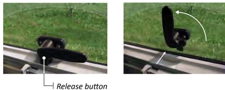
To open the window, unlatch the lever by pressing the release button and turn the lever to the left into the vertical position.
