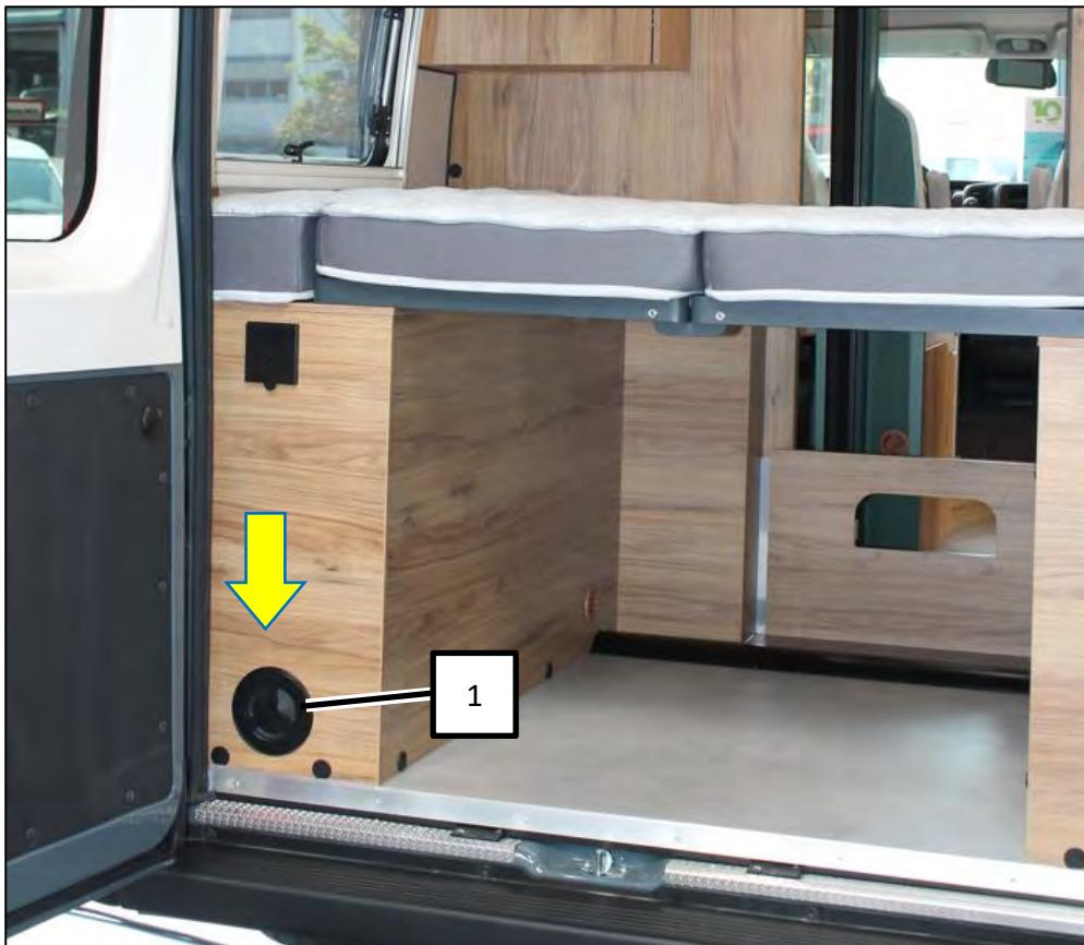
Access to the drain lever for the fresh water tank (sample illustration)
