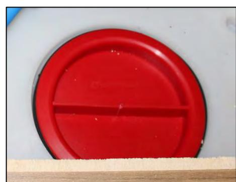
Screw-on cover for fresh water tank (sample illustration)
