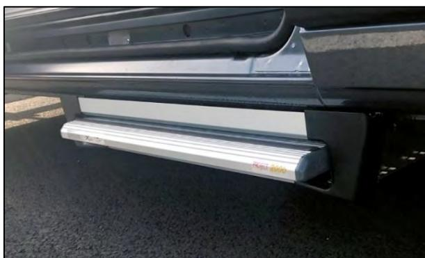
Your vehicle is equipped with an electric step for easy access to the living area.
