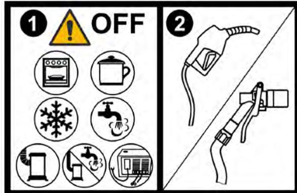
*Label "Close gas shut-off valves before refuelling"
