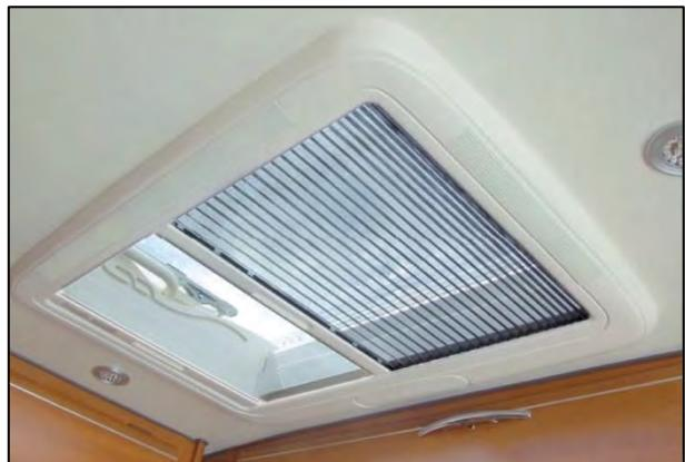
Insect screen roller blind on the roof light (sample illustration)
