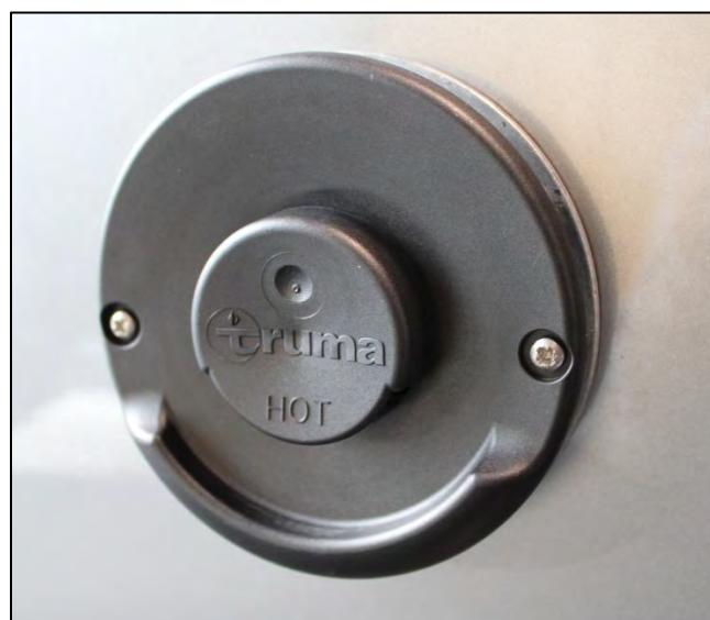
*Air intake/outlet element on the outside of the vehicle (sample illustration)*
