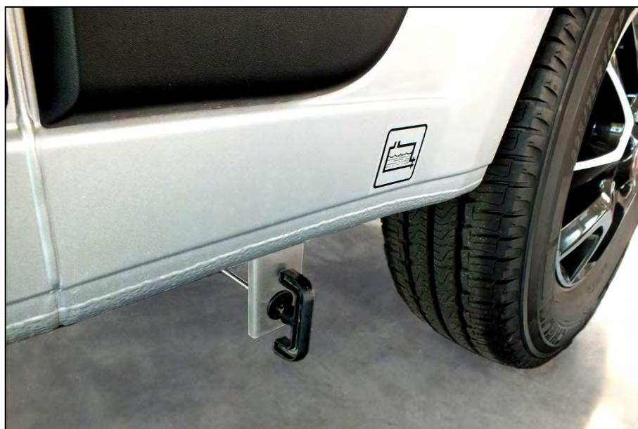
*Handle for draining the waste water tank*
