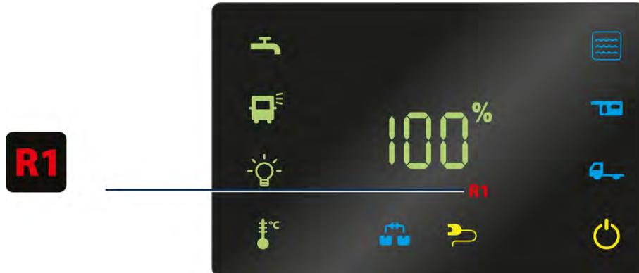
*Waste water tank warning signal (sample illustration)*
