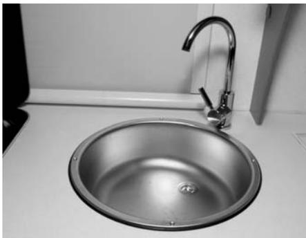
The sink of your Karmann motorhome is supplied with a mixer tap, which functions like a standard household tap. However, first make sure that the pump switch is on (see control panel, Page 6-1).
