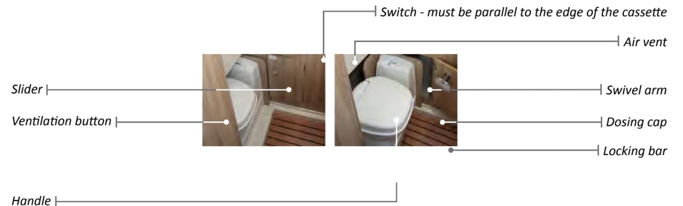
The cassette is accessible via a flap on the left-hand side of vehicle.
