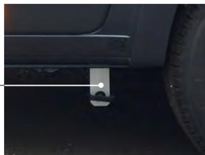
Handle to drain the waste water tank
