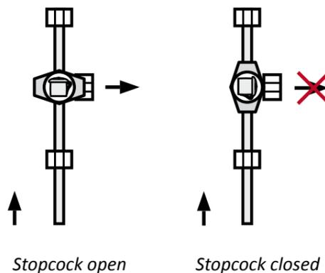
For putting the system into operation connect the main stopcock to the top cylinder. Once the main stopcock has been connected, turn the stopcock for a quarter of a turn to open the gas supply.
