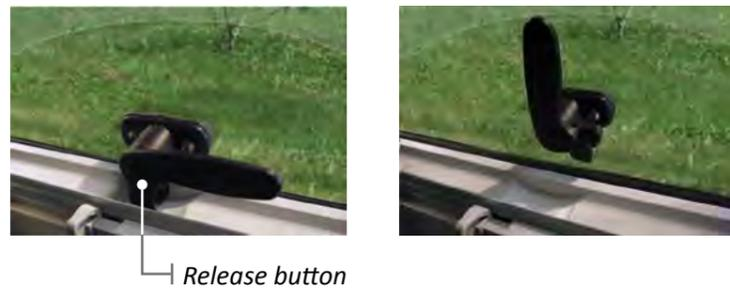
To open the window, unlatch the lever by pressing the release button and turn the lever to the left into the vertical position.
