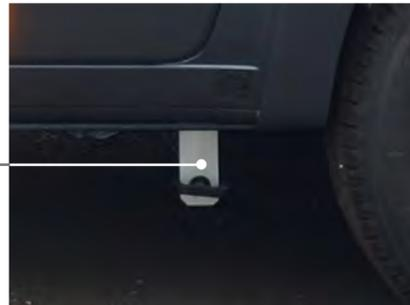
Handle to drain the waste water tank
