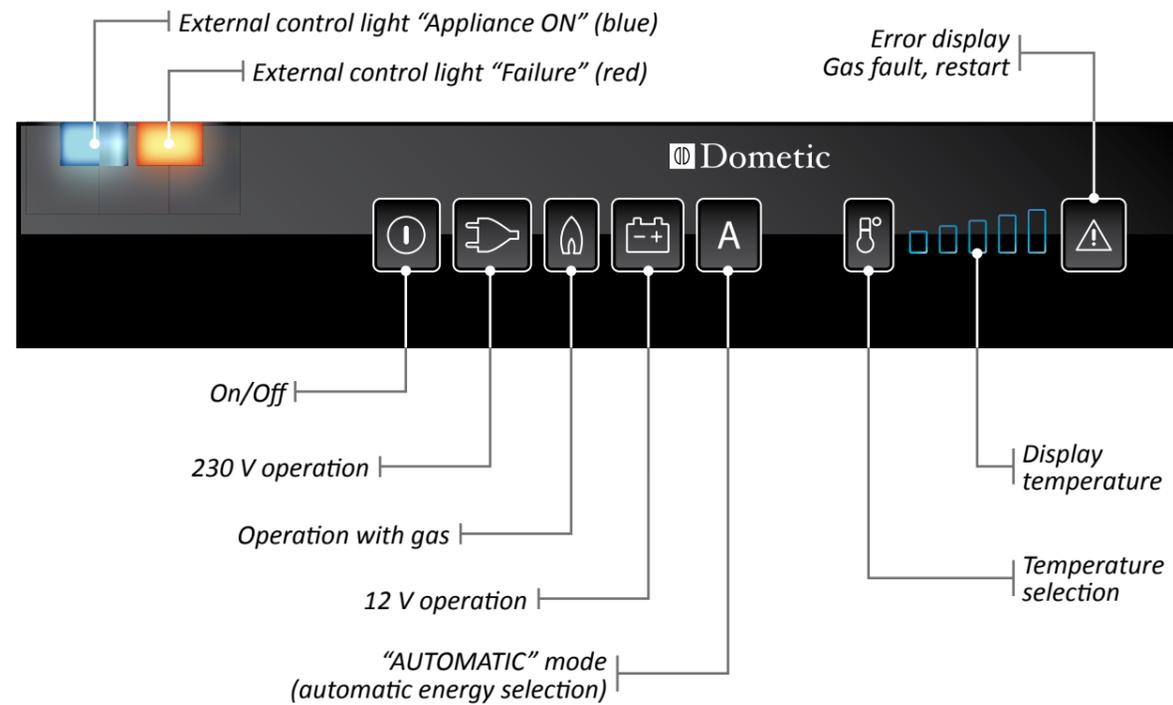
To turn the unit on or off, press and hold the button for 2 seconds.
