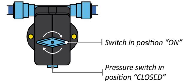
Turn the pump on at the control panel.
