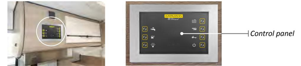
The control panel allows you to control various electric appliances in your vehicle and to check several parameters for the optimal use of the living room.
