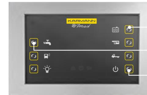
Control light for fresh water tank filling level
