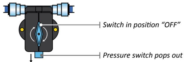
The water from the boiler is now drained to the outside via the drain valve. Place a container under the outlet to ensure that the boiler has been completely emptied (about 10 litres).
