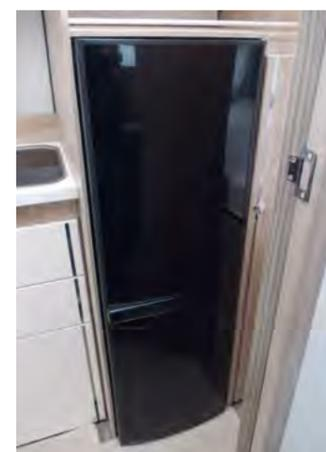
Your car is equipped with a refrigerator made by **Dometic** with **AES** (Automatic Energy Control System). This refrigerator can be operated by plugging it into the mains (230 V AC), with 12 V DC or with propane. Press MODE button to toggle between these types of energies.
