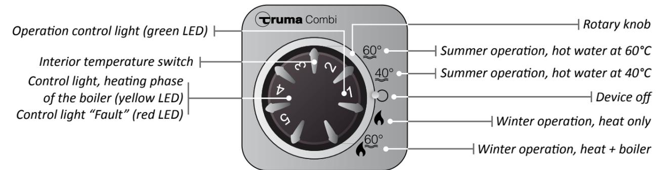
In order to switch on the power supply to the heater, the rotary knob must first be set to the mode for winter operation. The heating system can be operated either alone (without hot water production) or in combination with the boiler (with hot water production).
