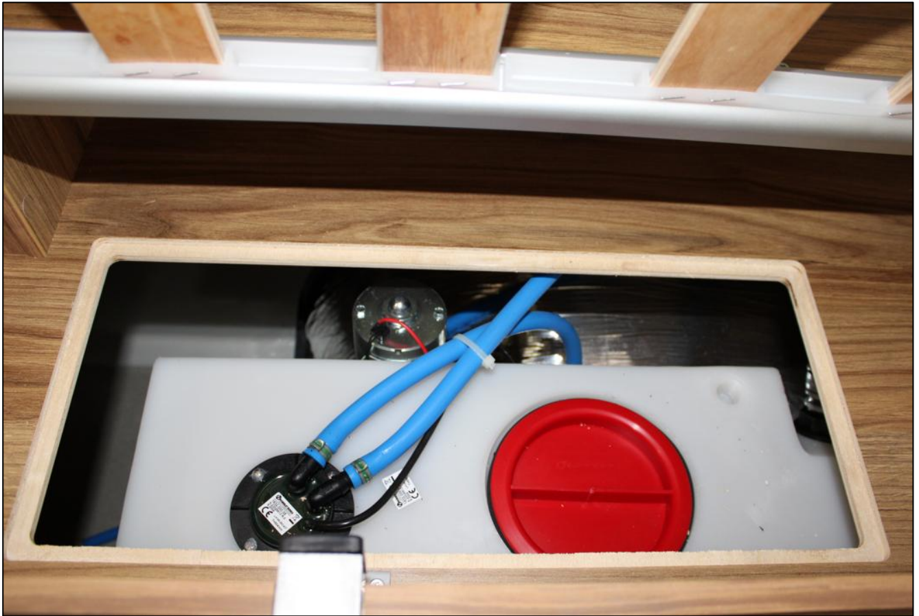
Fresh water tank in the bed base (for illustration purposes only)
