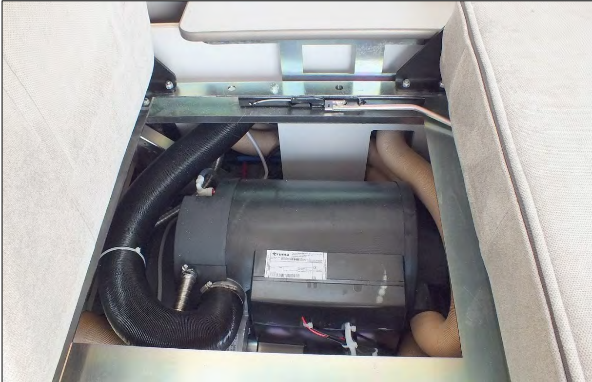
Heater in the seat compartment of the seat bench in the Dexter 550 (illustration purposes only)
