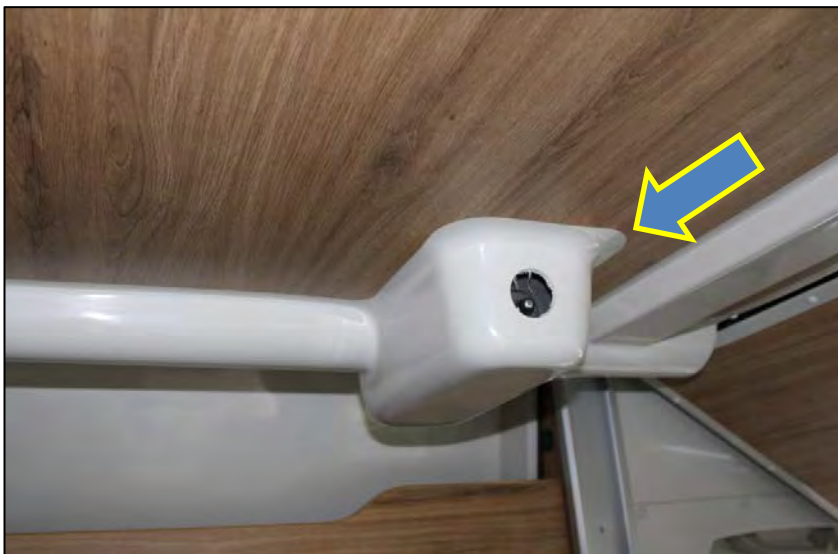
Access to the drive for the electric drop-down bed (illustration purposes only)
