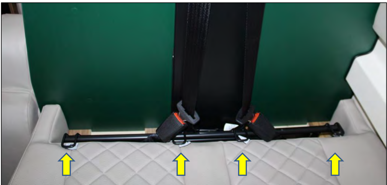
ISOFIX anchor point in the bench seat, backrest cushion removed (illustration purposes only)
