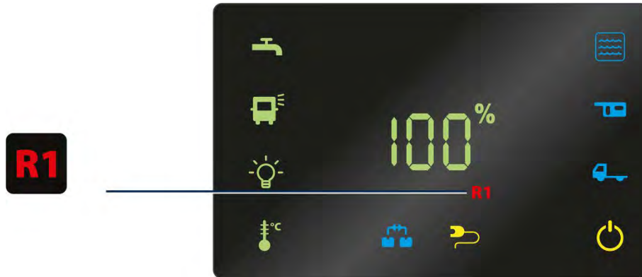
Waste water tank warning signal (illustration purposes only)
